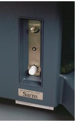
Integrated electronic gas blender can be controlled through the Central Control Monitor or locally.
