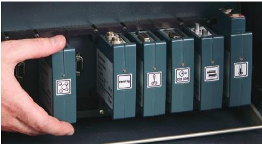
The Terumo System 1 can integrate up to 18 modules. These compact modules are plugged into the base of the system.
